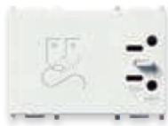
14290.AB 230 V~ shaver socket outlet, 50/60 Hz, with 20 VA isolating transformer, 230 V~ and 120 V~ outputs - 3 modules. Depth: 41 mm
