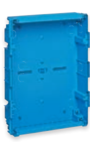
V53324 24-module flush mounting box (GW 650 °C) for masonry walls. Dim. 316x423x80 mm V53724 As above, for hollow walls
