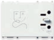
14290 230 V~ 50/60 Hz, with 20 VA isolating transformer, 230 V~ and 120 V~ outputs - 3 modules. Depth: 41 mm
