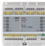
01470.1 Module with 9 inputs and 8 preprogrammed outputs for residential or hotel applications, N/O relay outputs 16 A 120-230 V~ 50/60 Hz programmable with function for lights, roller shutters with slat orientation, local control, 6 modules size 17.5 mm
