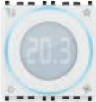
02971.B Home automation system dial thermostat for room temperature control (heating and air conditioning), 2- and 4-pipe system management, 3-speed and proportional fan coil control, class I temperature control device (contribution 1%) in ON/OFF mode, class IV (contribution 2%) in PID mode, can be interfaced with actuator with proportional analogue outputs 01466.1 to make a class V modulating room thermostat (contribution 3%), 1 input for electronic temperature sensor 20432, 19432 or 14432 or wired temperature sensor 02965.1, white LED backlighting
