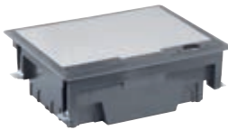
V54912.01 Floor mounting retractable turret with stainless steel cover for Eikon, Arké and Plana devices for installation on floating floors. Supplied with 2 mounting frames with 6 modules. Installation in screed with dedicated mounting box V54912
