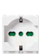
14210.AB SICURY 2P+E 16 A 250 V~ socket outlet, universal - 2 modules. Depth: 25 mm
