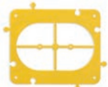
V71573 Mounting frame for installing boxes V71703 on the inside of the wall, yellow: •centring template; •coupling joint for mounting boxes in horizontal or vertical series
