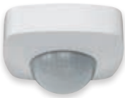
02690 Motion and presence detector, 360° for lighting 2000 W incandescent lamps, 10-1000 W CFL lamps, 100 W LED lamps, 220-240 V~ 50/60 Hz, for ceiling mounting
