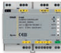
01465 HVAC controller for heating systems, 120-230 V~ 50/60 Hz, 3 inputs for PT100, PT1000 and NTC probes, 1 mixer valve control output, 1 output 0-10 V or (0)4-20 mA, 1 change-over relay output 16 A 230 V~, 6 modules size 17.5 mm
