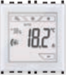
02951.B Touchscreen thermostat (heating and air-conditioning), 2 and 4 pipe system management, 3-speed and proportional fan-coil control, class I temperature control device (contribution 1%) in ON/OFF mode, class IV (contribution 2%) in PID mode, 1 input for flush mounting or wired NTC temperature sensor, RGB LED backlighting, can be interfaced with actuator with proportional analogue outputs 01466 to make a class V modulating room thermostat (contribution 3%) - 2 modules
