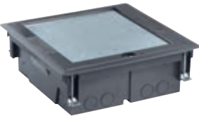
V54420 Floor mounting retractable 20-module turret with hollow cover for Eikon, Arké and Plana devices for installation on floating floors. Supplied with 4 mounting frames with 5 modules. Installation in screed with dedicated mounting box V54920
