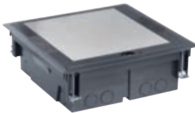
V54420.01 Floor mounting retractable 20-module turret with stainless steel cover for Eikon, Arké and Plana devices for installation on floating floors. Supplied with 4 mounting frames with 5 modules. Installation in screed with dedicated mounting box V54920
