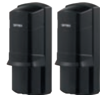
01743 Barrier kit consisting of TX/RX active infrared pair (AIR) with outdoor range of 60 metres, with 4 selectable channels to create a column barrier comprising several stacked detectors, IP65, 1 NO/NC 28 VDC 0.2A relay output for alarm, 1 NC 28 VDC 0.2A relay output to prevent false alarms due to adverse weather conditions (fog, rain, snow), 10.5-28 VDC power supply with 48 mA 12V surface, pole, column mounting, for outdoor use
