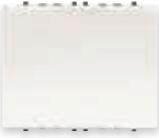
14463 Electronic badge switch, vertical pocket, relay output 4 A 120-230 V~ (NON SELV), 120-230 V~ 50/60 Hz, installation on 2-module or 2 central module mounting frames - 2 modules. Supplied without ISO card (badge) Depth: 20.5 mm
